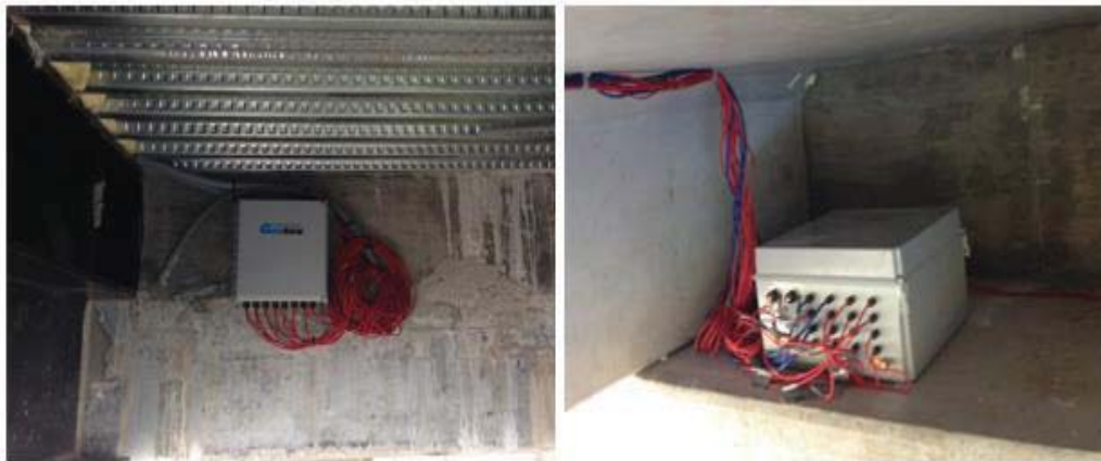
Figure 1.3: Data acquisition stations installed permanently below the Fate (left) and the Innovation (right) Bridge
