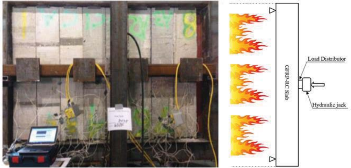
Figure 4.4: GFRP-RC slabs facing the vertical furnace
