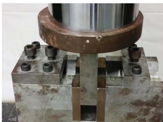
Figure 4.8: GFRP bars tested in transverse shear fixture
