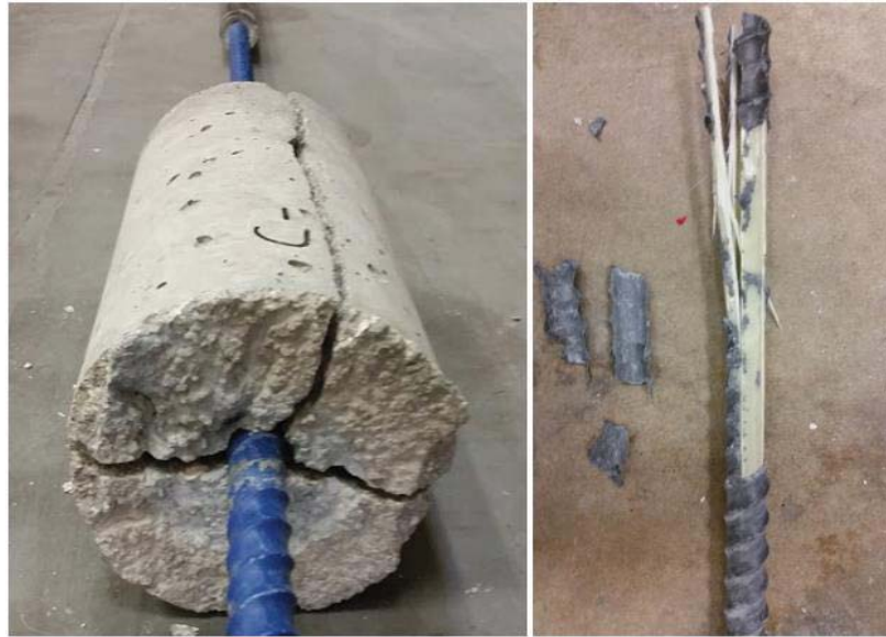
Figure 2.4: Concrete splitting (left) and peeling of the GFRP-H surface in samples with longer embedment length
