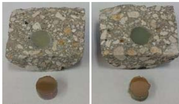
Figure 4.14: GFRP samples prior to SEM imaging: GFRP-A (left) and GFRP-C (right)
